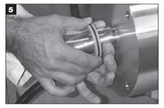
Slip one end onto the shaft by flaring the cylinder formed by the shim stock over the end of the shaft.
