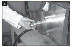
Align the end of the cylinder formed with the shim stock to the end of the shaft.
