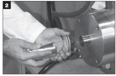
Use 0.005" thick brass shim stock cut to a length larger (approx. 1/4") than the circumference of the shaft. Roll the shim stock and place into the inside of the seal.
